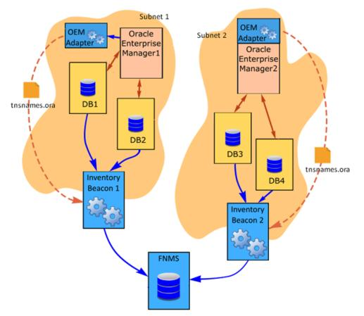
The above diagram shows Subnet 1 and Subnet 2. Subnet 1 is assigned to Inventory Beacon 1 and Subnet 2 is assigned to Inventory Beacon 2. Each subnet contains:
