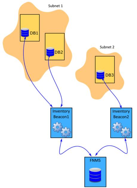
The above diagram shows three database servers, two on Subnet1 and one on Subnet2. The Subnet1 is assigned to Inventory Beacon1 and Subnet2 is assigned to Inventory Beacon2. Note that in this diagram, DB1 and DB2 are running versions of Oracle Database compatible with the same OLEDB driver, as discussed in Direct Collection of Oracle Inventory; separately, DB3 may also be compatible, or may require a different version, which may be the reason that it is managed by a separate inventory beacon.
