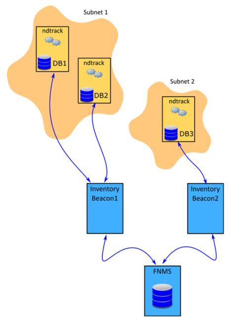
The above diagram shows three database servers, two in Subnet1 and one in Subnet2. The Subnet1 is assigned to Inventory Beacon1 and Subnet2 is assigned to Inventory Beacon2. Each inventory beacon can connect to the Oracle server(s) in its assigned subnet. All the prerequisites outlined in Zero-footprint Collection of Oracle Inventory are satisfied.
