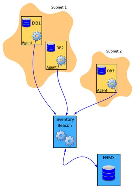
The diagram shows three database servers, two in Subnet1 and one in Subnet2. An instance of FlexNet Inventory Agent has been installed on each of these database servers. The inventory beacon has been assigned to cover both of these subnets and can connect to every Oracle server. All the prerequisites outlined in Agent-Based Collection of Oracle Inventory are satisfied.
