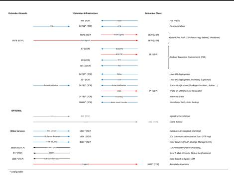
The network ports vary depending on the modules and components applied.
