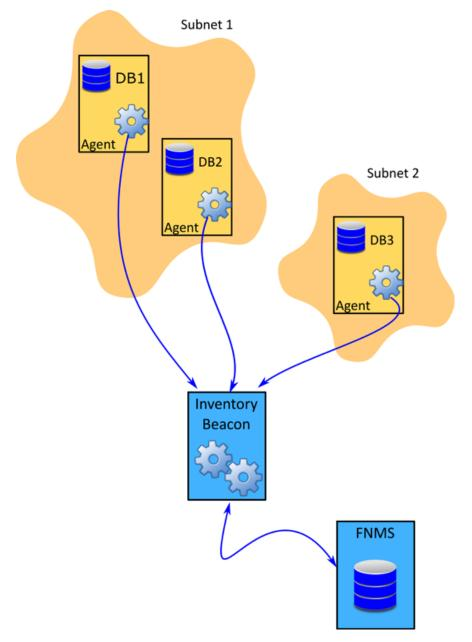
The diagram shows three database servers, two in Subnet1 and one in Subnet2. An instance of FlexNet inventory agent has been installed on each of these database servers. The inventory beacon has been assigned to cover both of these subnets and can connect to every Oracle server. All the prerequisites outlined in Agent-Based Collection of Oracle Inventory are satisfied.
