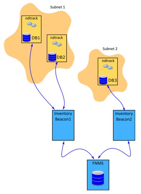
The above diagram shows three database servers, two in Subnet1 and one in Subnet2. The Subnet1 is assigned to Inventory Beacon1 and Subnet2 is assigned to Inventory Beacon2. Each inventory beacon can connect to the Oracle server(s) in its assigned subnet. All the prerequisites outlined in Zero-footprint Collection of Oracle Inventory are satisfied.
