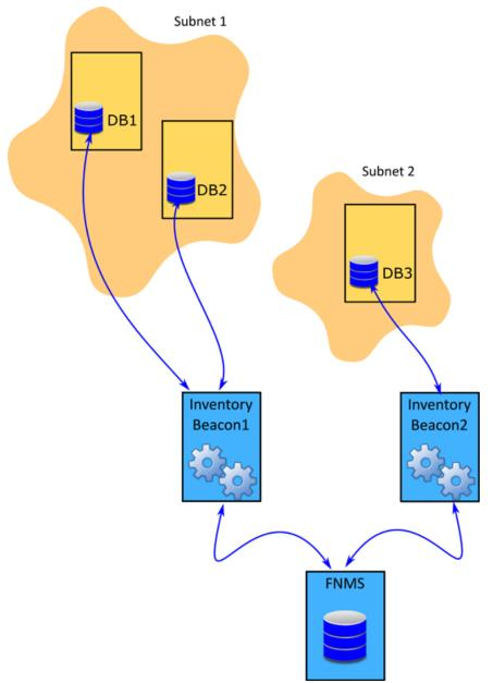
The above diagram shows three database servers, two on Subnet1 and one on Subnet2. The Subnet1 is assigned to Inventory Beacon1 and Subnet2 is assigned to Inventory Beacon2. Note that in this diagram, DB1 and DB2 are running versions of Oracle Database compatible with the same OLEDB driver, as discussed in Direct Collection of Oracle Inventory; separately, DB3 may also be compatible, or may require a different version, since it is already managed by a separate inventory beacon.
