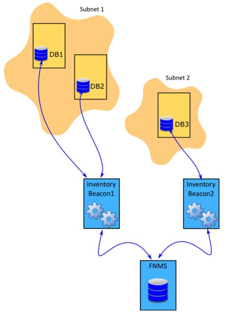
The above diagram shows three database servers, two on Subnet1 and one on Subnet2. The Subnet1 is assigned to Inventory Beacon1 and Subnet2 is assigned to Inventory Beacon2. Note that in this diagram, DB1 and DB2 are running versions of Oracle Database compatible with the same OLEDB driver, as discussed in Direct Collection of Oracle Inventory; separately, DB3 may also be compatible, or may require a different version, since it is already managed by a separate inventory beacon.
